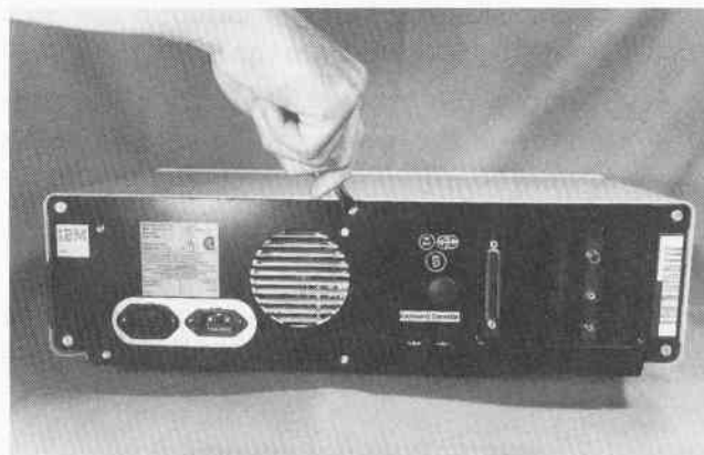
Fig. D-1. Remove these screws to disassemble the IBM PC.
